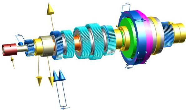
Individual load spectra can be assigned to every force element. The shaft geometry can be exported to a range of 3D CAD systems for further processing.
