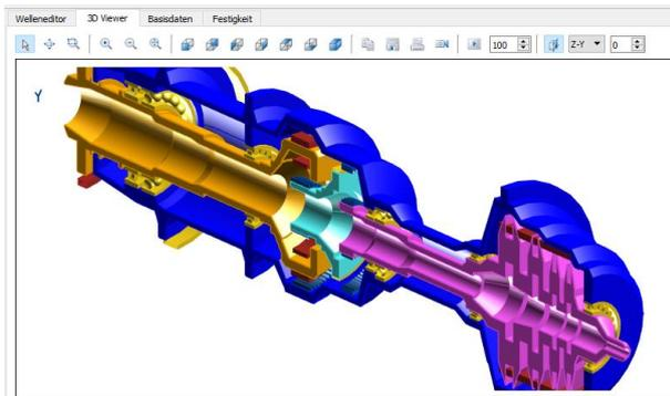
Shafts can now also be easily selected and moved by a mouse click. For complex systems made of different shafts, this feature makes it easier to move single shafts in the foreground or in the background.
