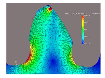
An asymmetrical tooth form can be calculated for all cylindrical gear configurations. This option must be activated in the module-specific settings. Either the modified ISO 6336 or VDI plastic methods can then be used to evaluate strength.
