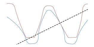
Alternatively, asymmetric gears can be defined also by defined in the tab 'Tooth form' by reading in a DXF file.
