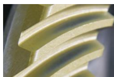
Figure 34. Typical contact pattern with tester
