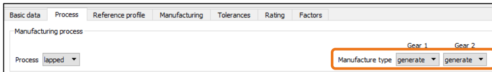
Figure 22. «For generated gears» and «Made by form cutting» manufacturing types
