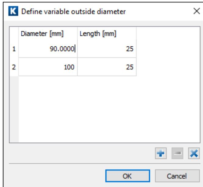
Figure 11. Defining a hub with variable outer diameter
