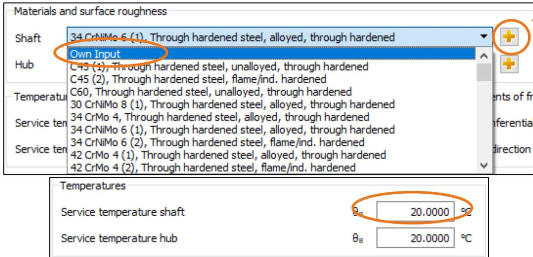
Figure 14. Inputting your own material (in particular coefficient of thermal expansion) and operating temperature
