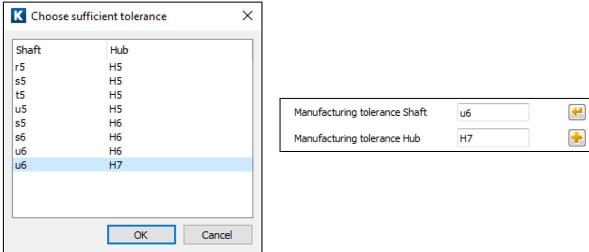
Figure 4. Selecting and transferring a tolerance pair
