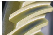
Figure 34. Typical contact pattern with tester
