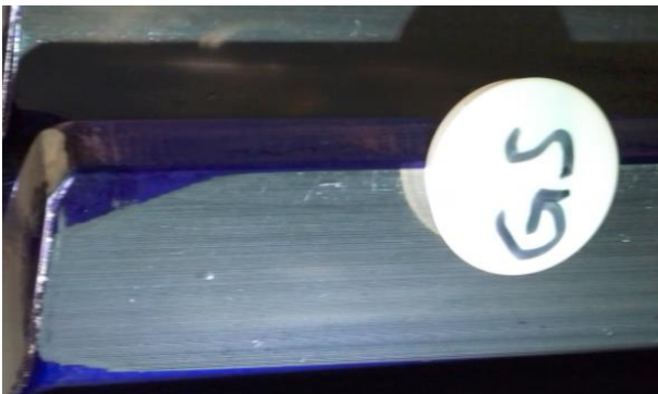
Example: Rating of 3MW wind gearbox components for certification along GL guideline, test witnessing, contact pattern assessment
