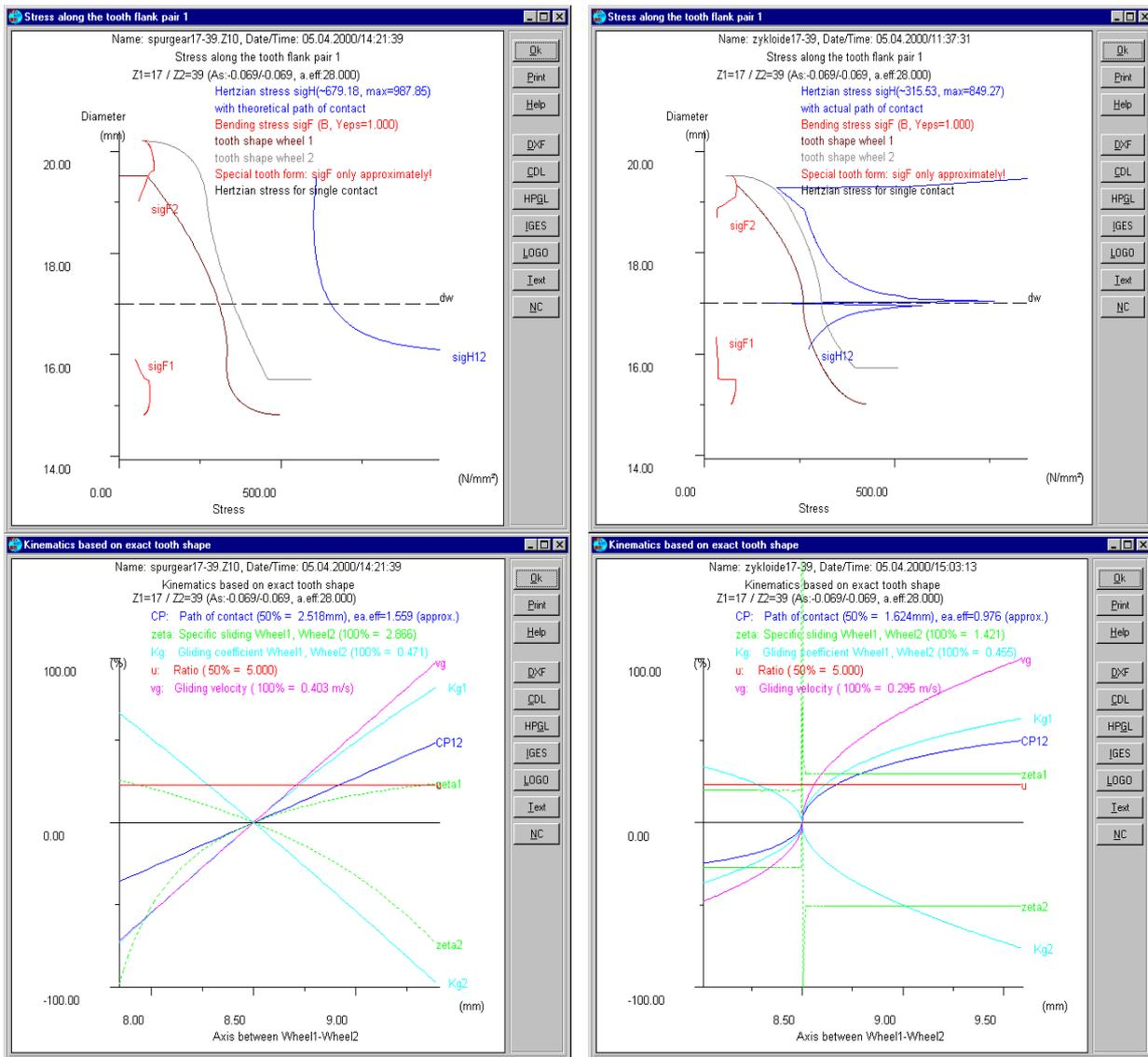
Figure 0-1 Comparison between the Hertian-pressure and the kinematic conditions of an involute gear with a cycloid wheel pair (number of teeth 17 : 39)
