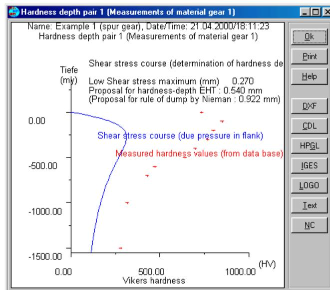
Figure 0-1 Determination of the hardness depth (Hoop stress perpendicular to the tooth surface, points of hardness measurements)
