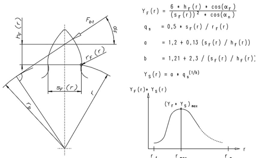
**Figure 0-1 Derivation of the tooth root stress at any location of the root between Y<sub>F</sub>(r) and Y<sub>S</sub>(r)**
