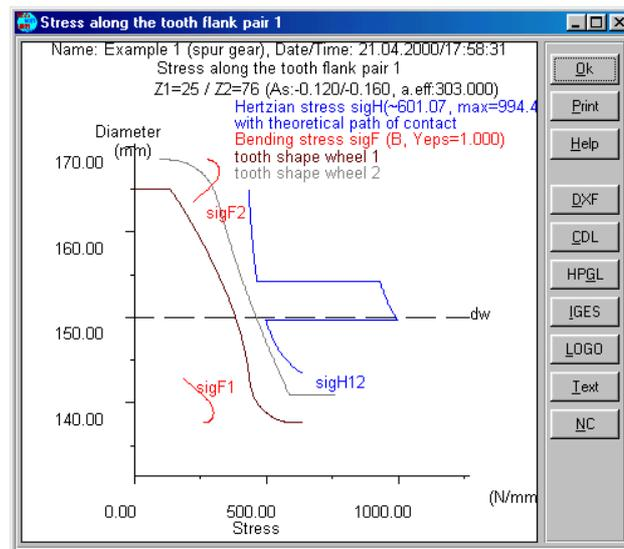
**Figure 0-2** Tooth root stresses (and Hertzian-pressure), calculated on the base of the actual tooth form and the meshing conditions.
