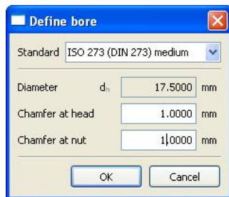
Figure 2.4-2: Definition of the clamped parts
