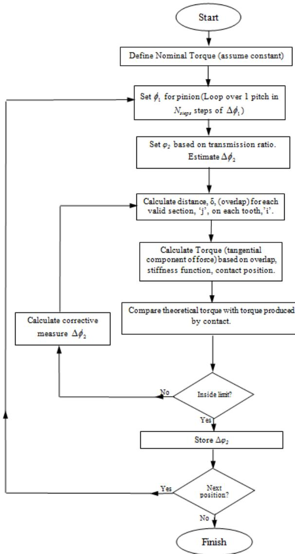
Fig. 1: tooth contact analysis according to Peterson
