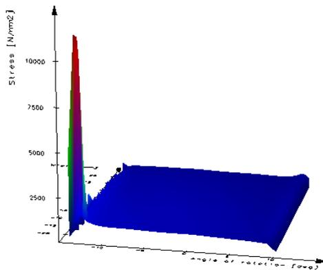
Fig. 8a: high pressure peak due to no tip rounding
