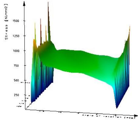
Fig 8b: much lower pressure with tip rounding 0.5mm
