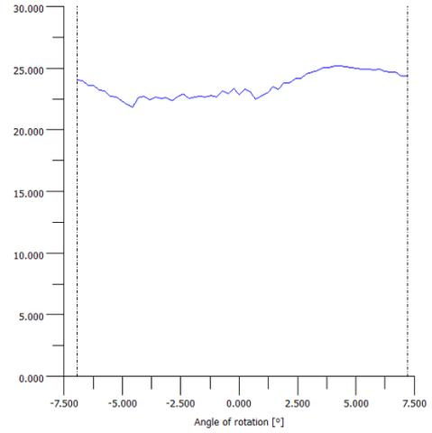
Fig 6b: KISSsoft 04-2010 calculates slightly lower tooth contact stiffness
