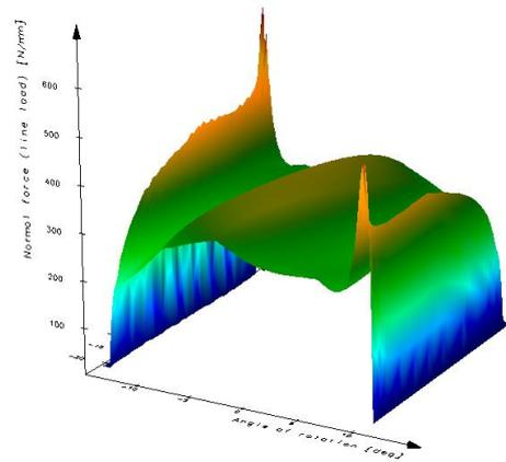
Fig 5b: KISSsoft 04-2010 shows higher normal forces (line load) at start and end of contact
