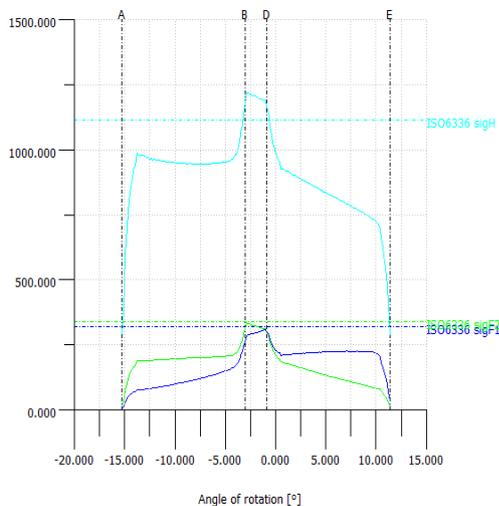
Fig. 7a: previous releases consider load distribution factors in tooth contact analysis
