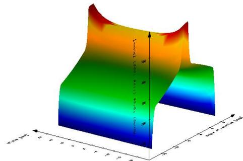
Fig 4b: KISSsoft 04-2010 shows the increased normal force (line load) at edges of contact area
