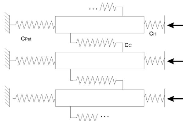
Fig. 2: stiffness model according to Peterson and KISSsoft Release 04-2010
