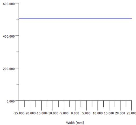
Fig. 4a: previous KISSsoft releases shows constant normal force (line load) over face width
