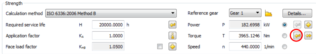
Figure 4.10 Calculating maximum transmissible torque
