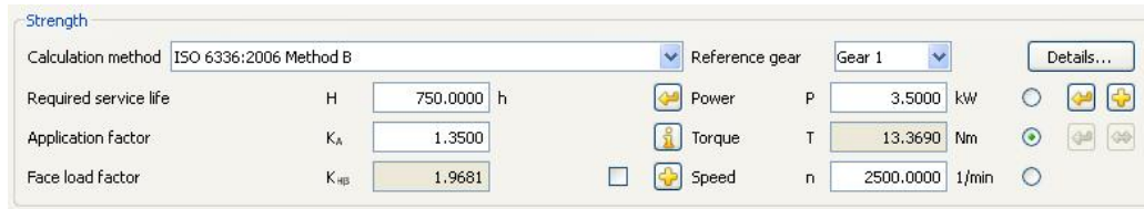
Figure 2.7 Input window – "Basic data" tab, Strength group
