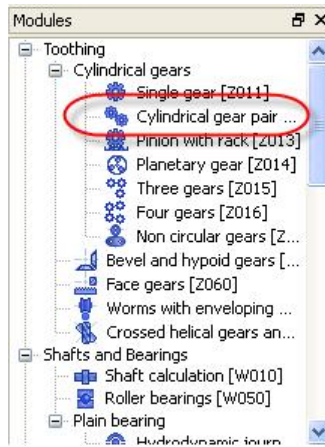
Figure 2.2 Calling cylindrical gear calculation
