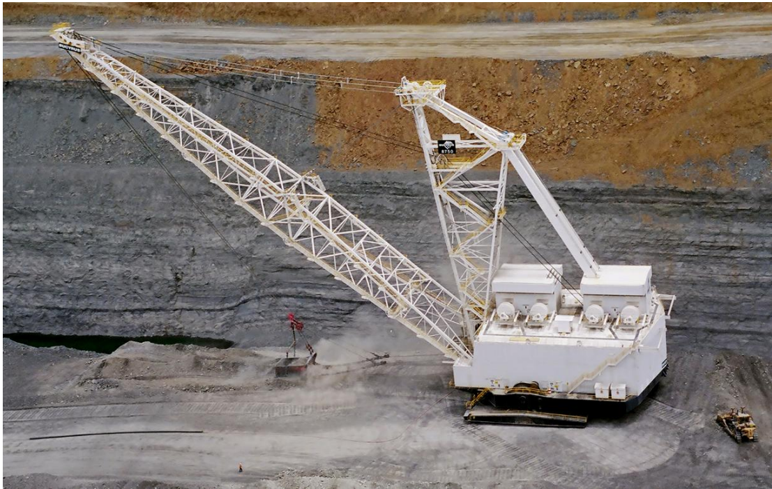
Figure 1 Surface mining dragline with the drives used in the analysis (photo BUCYRUS®, USA)
