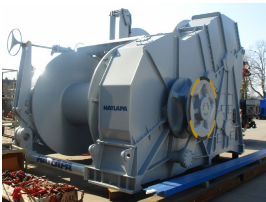
Figure 2.4-2 Final machinery with gearbox enclosed on right side of winch
