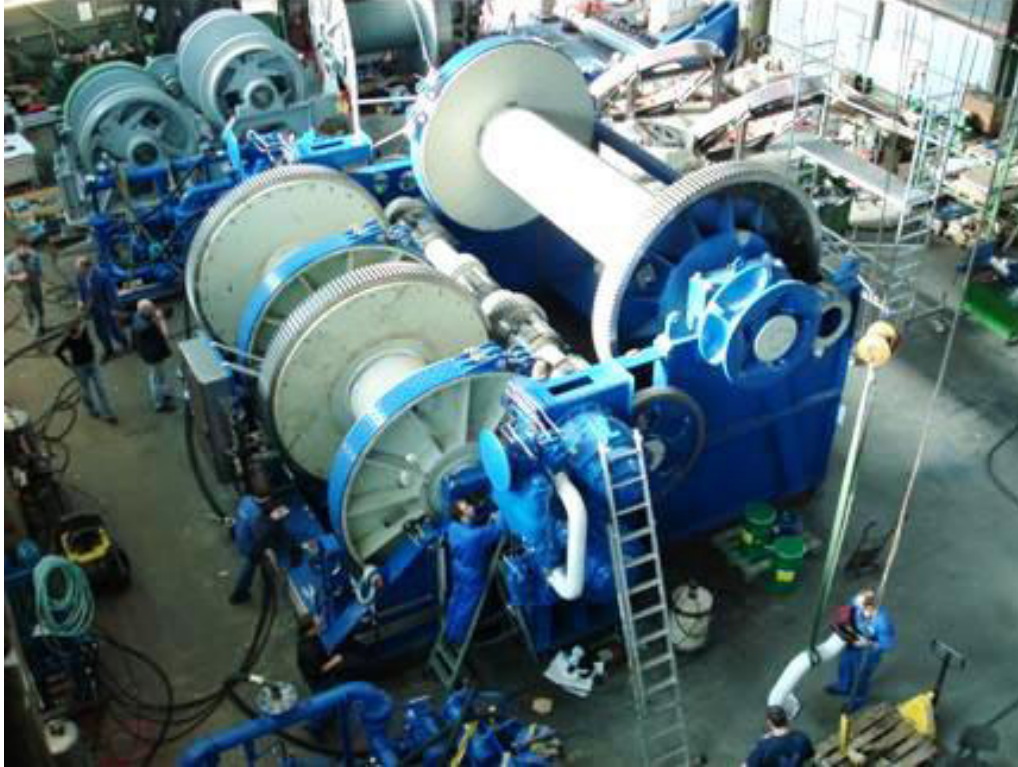
Figure 1.2-1 Typical deck machinery built at HATLAPA, including machinery components like gears, shafts, bearings analysed with KISSsys and KISSsoft; HATLAPA
